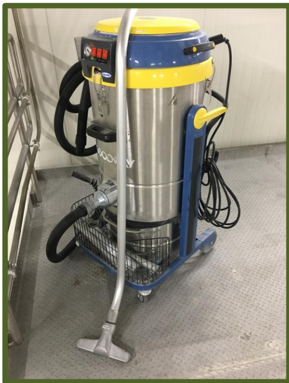
Figure 30. Dedicated HEPA filtered vacuum cleaners.
