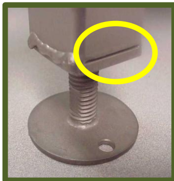
Figure 21. Hollow square tubing not hermetically
