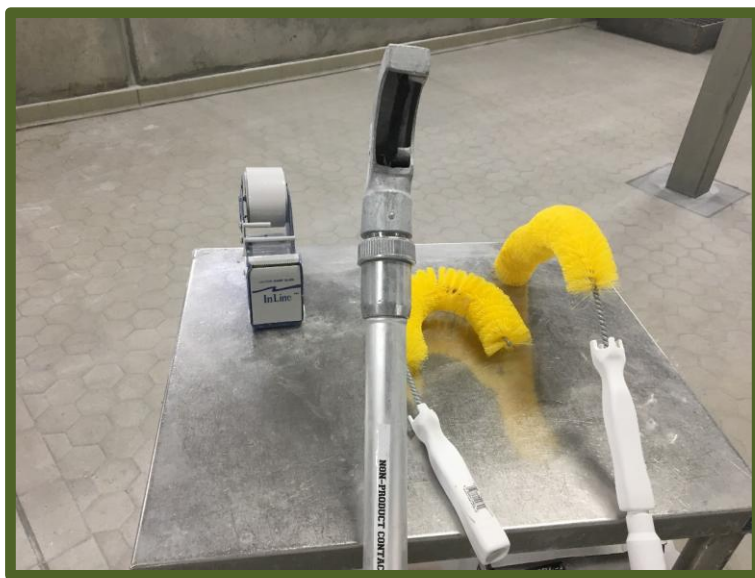
Figure 31. Overhead pipe exterior cleaning tools.
