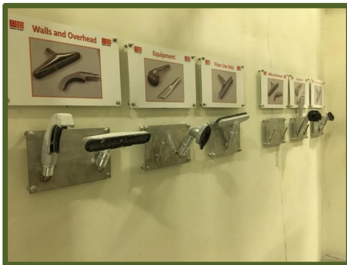
Figure 33. Vacuum attachments designed by shape rather than by color
