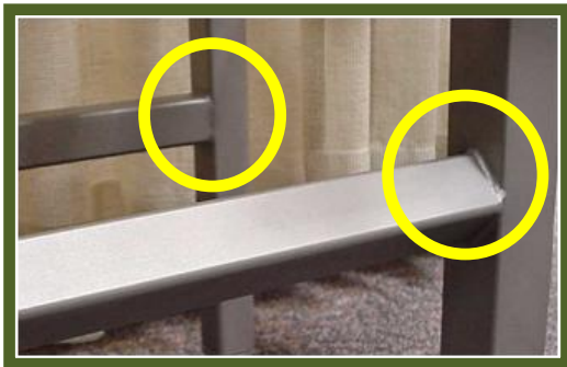
Figure 19. The square tubing on the left will accumulate soil on the flat horizontal surface. By rotating 90°, or using round tubing, flat surfaces are minimized.
