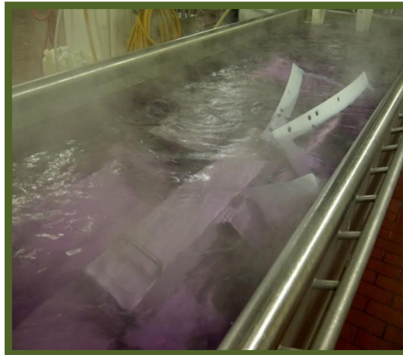
Figure 28. Equipment must be fully submerged for appropriate cleaning.
